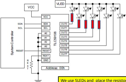
We use 5LEDs and place the resistors in series with the LEDs. Vf of LED is 2.8~3.1V.
