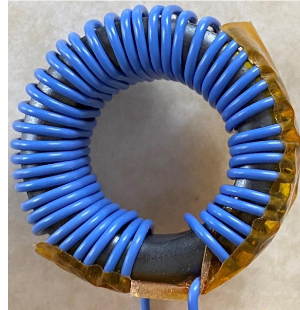
Inductor #2: Homemade by using toroid core Würth PN: 7427015 and 43 turns of single layer winding. Inductance measured at 1.39mH @ 300kHz.
