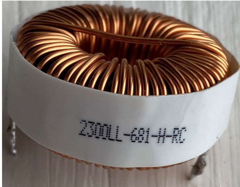
Inductor #1: Bourns PN: 2300LL-681-H-RC, 680uH Built by using toroid core, single layer winding. However, some amount of winding overlapping is visible.
