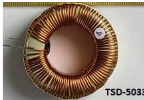
New toroidal PFC inductor (L2) w/o overlapping windings 750uH @ 8A
