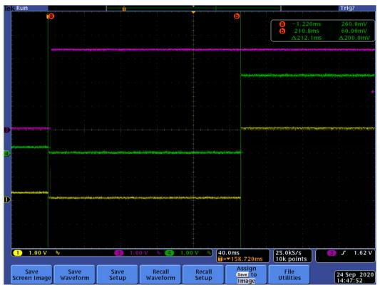
In above figure, we can see TPS3809 RESET signal is correct with 1kohm series resistor
