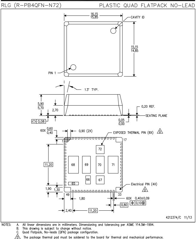
The package thermal pad must be soldered to the board for thermal and mechanical performance.
