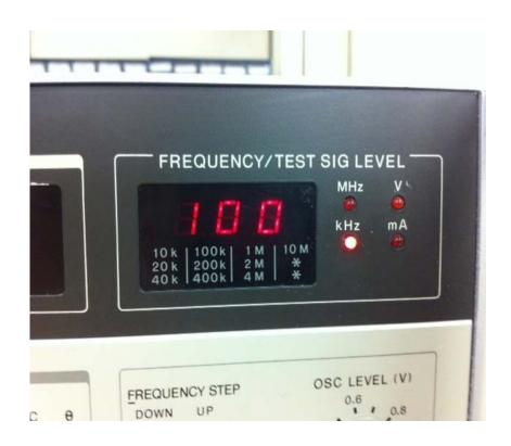
**Step 01:** Set the tuning frequency to 100KHz
