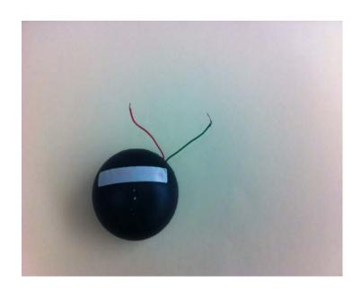
**Step 03:** Measure the inductance of the secondary coil away from transmitter pad and made in final configuration inside the case with shields and battery in place.
