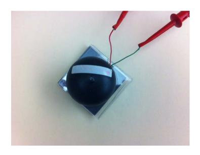
Step 05: Measure the inductance of the secondary (made in final configuration inside the case with shields and battery in place) when placed on transmitter pad. Secondary Coil and the center of the primary Shielding shall be aligned.
