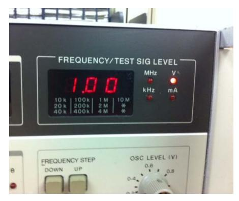
**Step 02:** Set the tuning voltage to 1-V RMS
