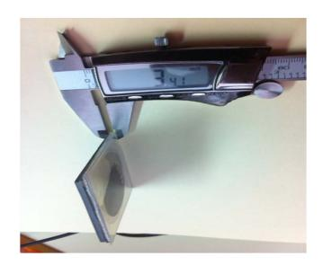
The distance from the Receiver Interface Surface to the primary Shielding is 3.4 mm.
