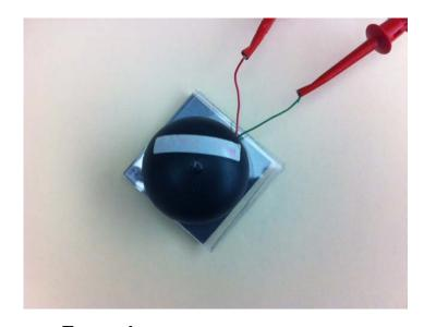
**Example:** Secondary coil (made in final configuration inside the case with shields and battery in place) when placed on transmitter pad. Secondary Coil and the center of the primary Shielding shall be aligned.
