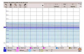
C1: 5Vout [100mV/div], C2: T1 primary current [500mA/div], C3: FB pin voltage [1V/div], C4: LL/SS pin voltage [1V/div]
