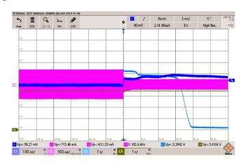
The momentary dip change seen before the improvement is no longer observed in the LL/SS pin waveform.
