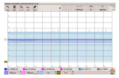
C1: 5Vout [100mV/div], C2: T1 primary current [500mA/div], C3: FB pin voltage [1V/div],
