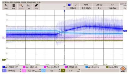
When the 5V output suddenly changed load, a momentary dip that was thought to be due to noise was observed in the LL/SS pin waveform.
