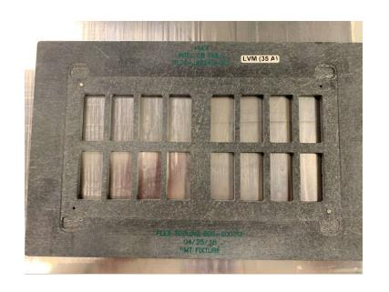
This is a BLR test board with passive on bottom side of the PCB close to the edge. The reflow fixture was to protect those passive mounted by the first reflow.
