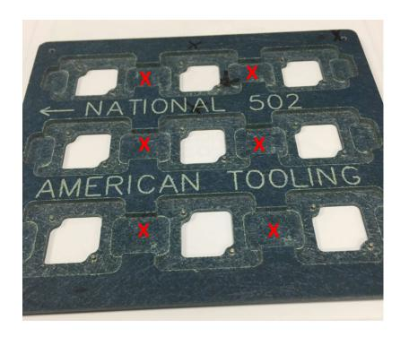
"X" were locations where components mounted during first reflow. They were protected by this fixture during second reflow.
