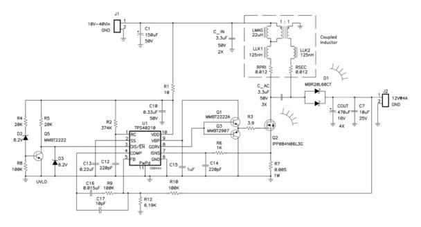
Figure 4: 12V@4A SEPIC converter schematic.
