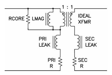
Figure 3: Non-ideal coupled inductor model.
