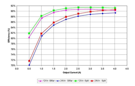
Figure 9: A loosely-coupled SEPIC provides better efficiency.
