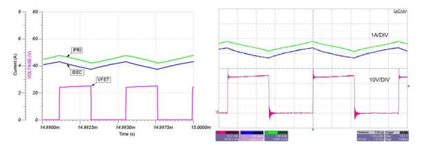
Figure 6: Leakage inductance produces well-behaved inductor currents. Simulation (left) and actual (right).
