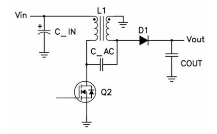
Figure 1: The basic coupled inductor SEPIC converter.
