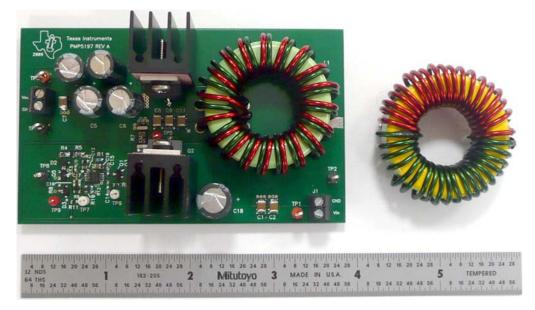
Figure 8: Evaluation hardware with tightly-coupled (left) and high-leakage split-winding inductors (right).
