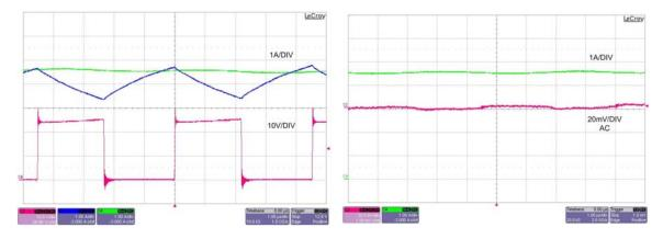
Figure 7: Ripple current is steered to the output, minimizing input ripple. inductor ripple currents (left) and input ripple voltage (right).
