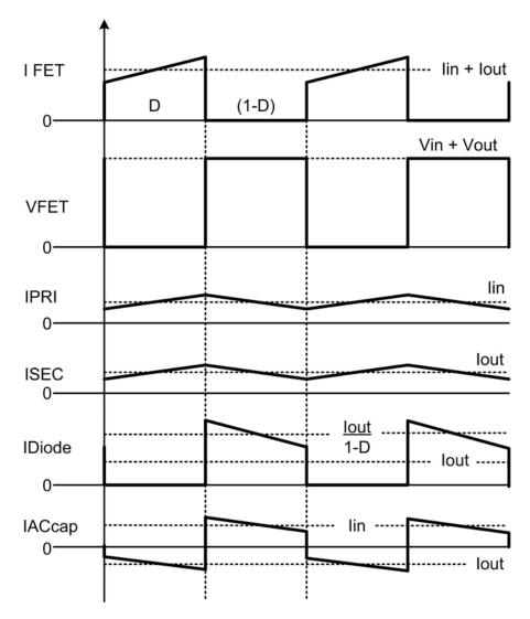
Figure 2: Key waveforms for a continuous conduction mode SEPIC.
