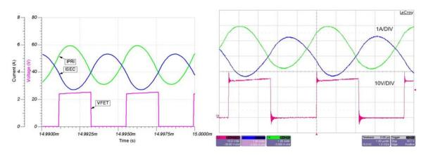
Figure 5: Inductor ripple currents for tightly-coupled magnetics may be much larger than expected. Simulation (left) and actual (right).
