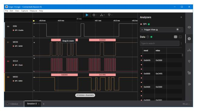
Step 2: Read STATUS register (Address = 0x01). According to datasheet this should clear SPE.
