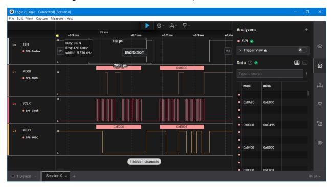
Step 4: Read STATUS register again ...the response frame is 0xE001 so the SPE flag is set in the response frame and the data portion also indicates and active SPI error condition.
