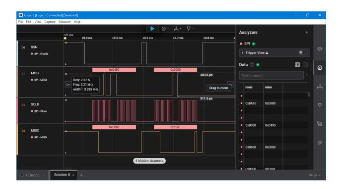
Step 3: Read ThermWarnLimit register (Address = 0x02). If the previous write operation was successful we should get back 0x96 in the datafield of the response frame.
