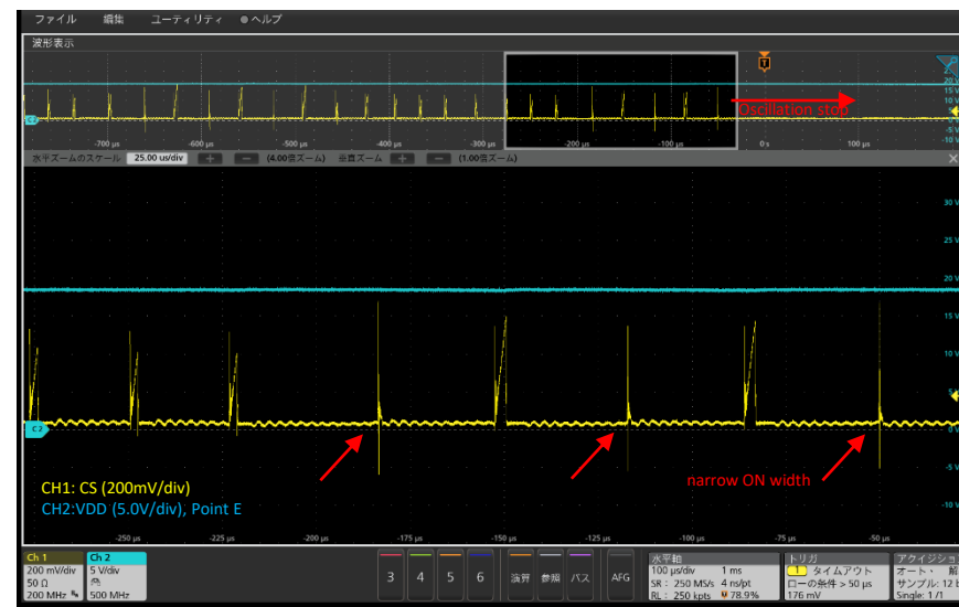
Fig.4 : CS pin (Point B) waveform just before oscillation stops (C25 uninstalled (0 pF))
