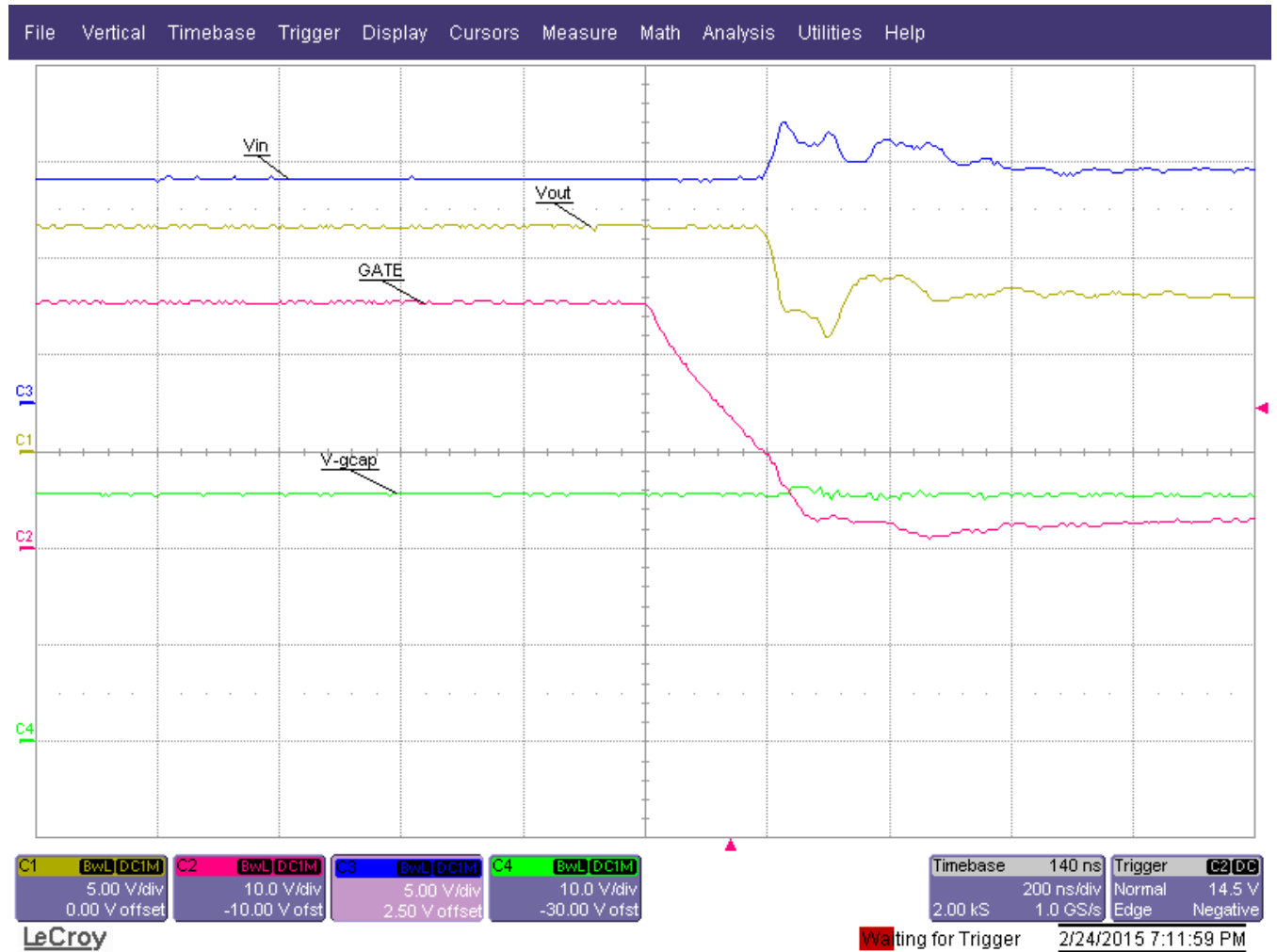
Figure 2. GATE Transient Response Characteristic: 1k \Omega resistor in series with C_{GATE} = 0.1\mu F
