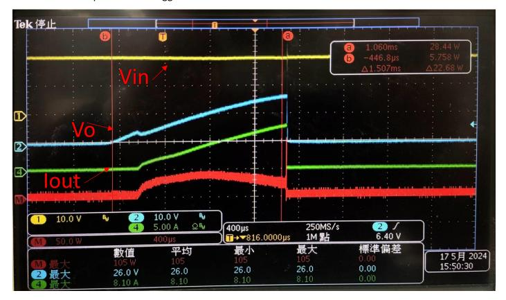
Is the device showing good test result in startup with Enable i.e. Vin is high and EN is low. You pull EN high and see if the device can startup. On EVM, to test this you need to press S1 switch and later release the switch to pull EN high.
