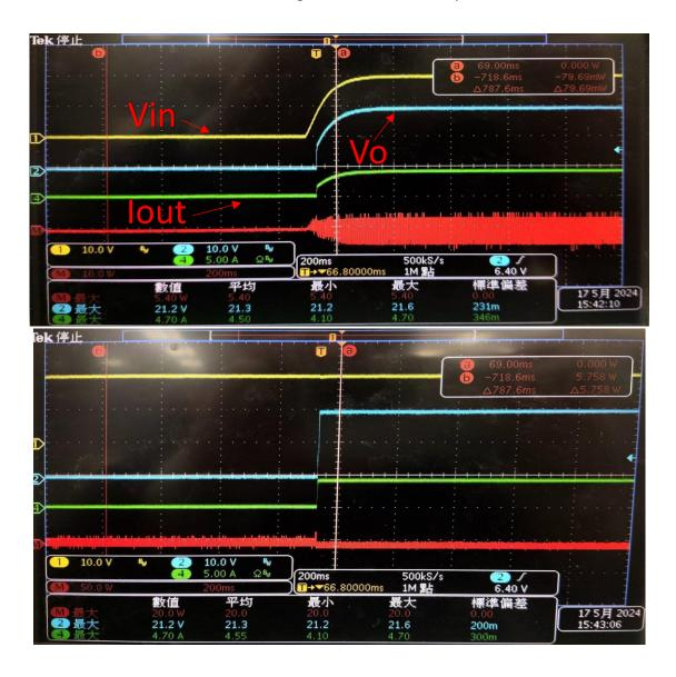
Test items3.CR Mode R:4 $\Omega$  (I=5A) , Vin 20V  $\circ$  PASS
