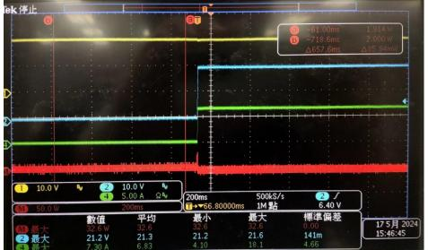
Test items5.CR Mode R:2  $\Omega$  (I=10A) , Vin 20V  $\circ$  FAIL
