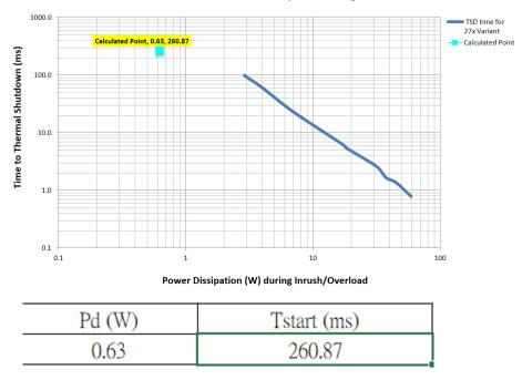
Thermal Shutdown Time Vs. Power Dissipation during Inrush/Overload
