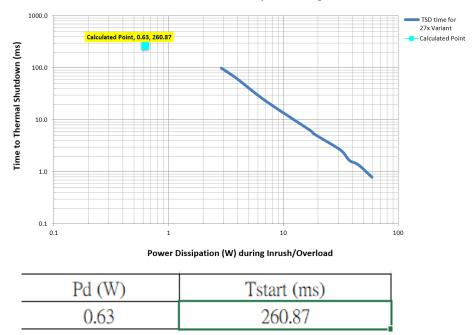
Thermal Shutdown Time Vs. Power Dissipation during Inrush/Overload
