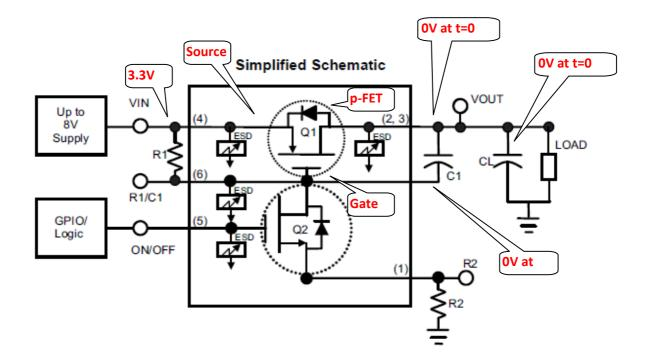
p-FET Vgs = -3.3V at t=0 => it conducts! Waveforms:
