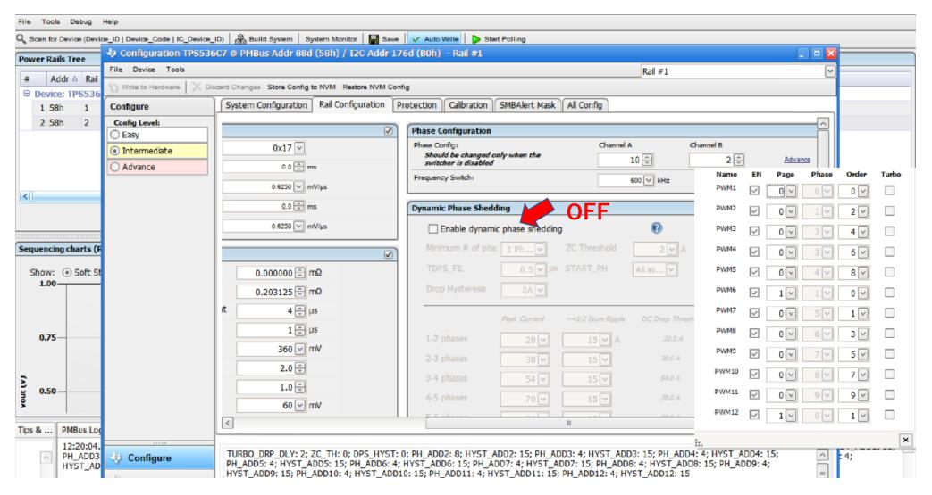
Current Config. Tab on 10 phase operation (no out put No.6 PWM and No.12 PWM) This "Advance" Order is this 10 phase operation situation.
