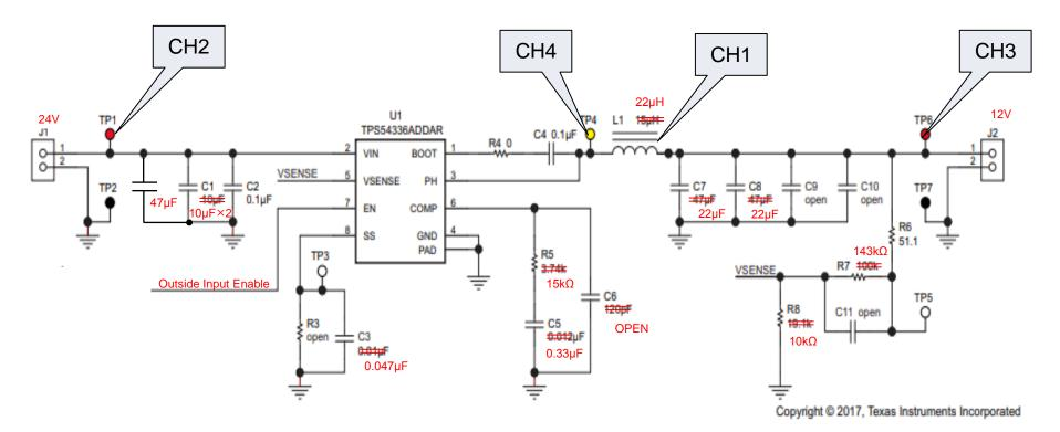
Figure 18. TPS54336AEVM-010 Schematic
