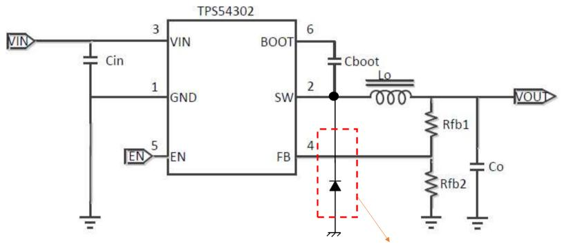
If the internal MOSFET does not have a diode, does it need to mount an external diode to protect the MOSET?
