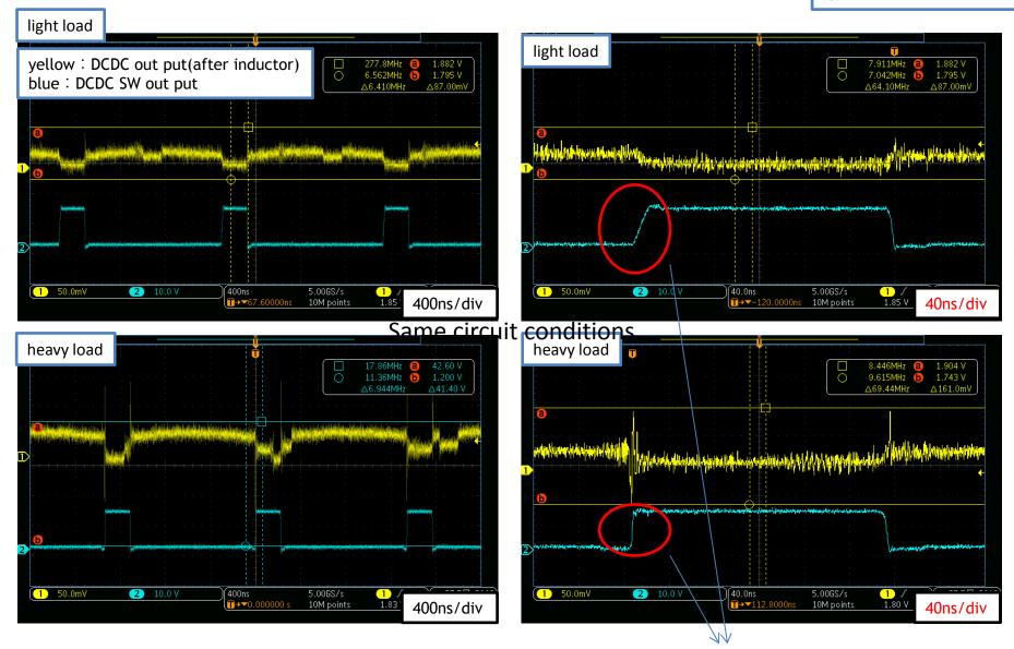
SW wave form slew rate is different in light load and heavy load conditions.
