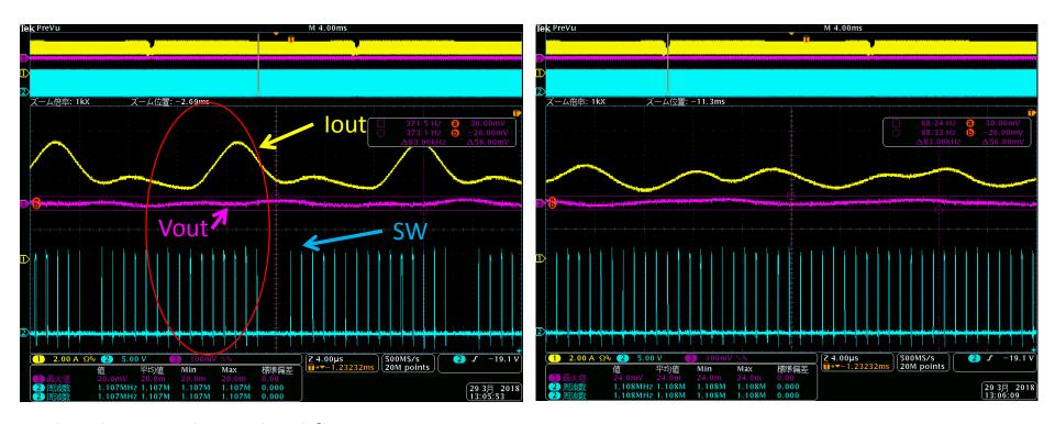
Pulse skipping due to load fluctuation.
