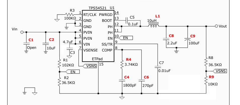
① Please refer to the datasheet section 'Enable and Adjusting Under-Voltage Lockout' for details on UVLO resistor calculations.
