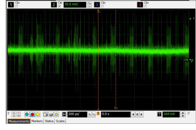
VIN= 14,5 V V LED+=13,7 V PWM= 0% V FB= 30/40mV I LED= 0,04/10R= 4mA PWM= 0%
