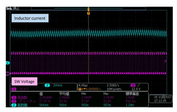
Vin=8V, Fsw=2MHz by SYNC pin
