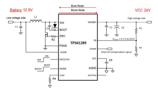
Buck Mode (normal operation / charged mode) VHIGH 24V battery charge 12.8V // charging current 60mA
