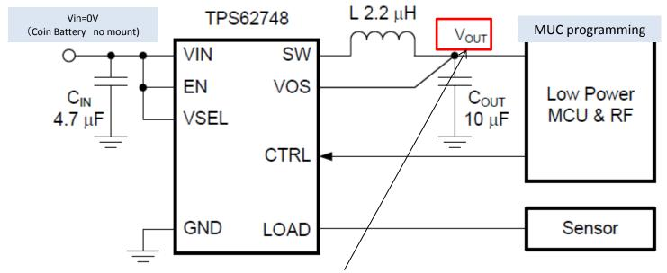
Customer to set up the MCU added to the voltage(1.8V) from outside source.
