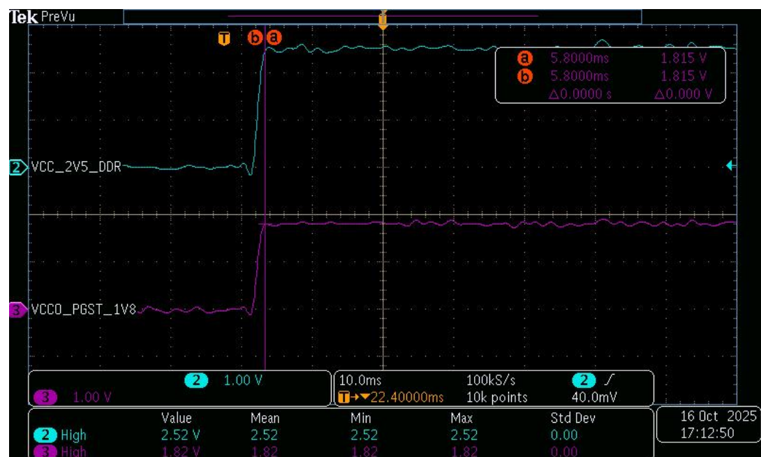
Figure 4: VCC_PGST_1V8 is generated from LDO1 at LOUT1 [Pin 31] is 1.8V
