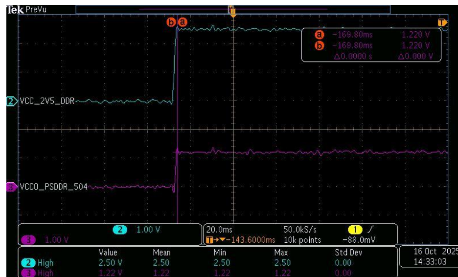
Figure 1: VCCO_PSDDR_504 is generated from Buck 1 at LX1 [Pin 26] is 1.2V
