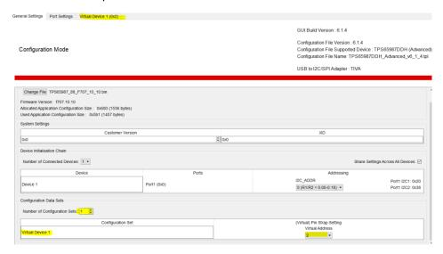
Go to the virtual device and remove all the registers by going to "Adjust Registers" and de-selecting all registers.
