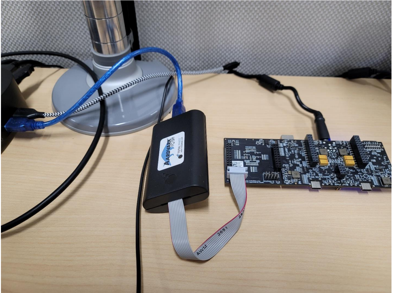
Figure 1: EVM Setup with Aardvark Adapter
