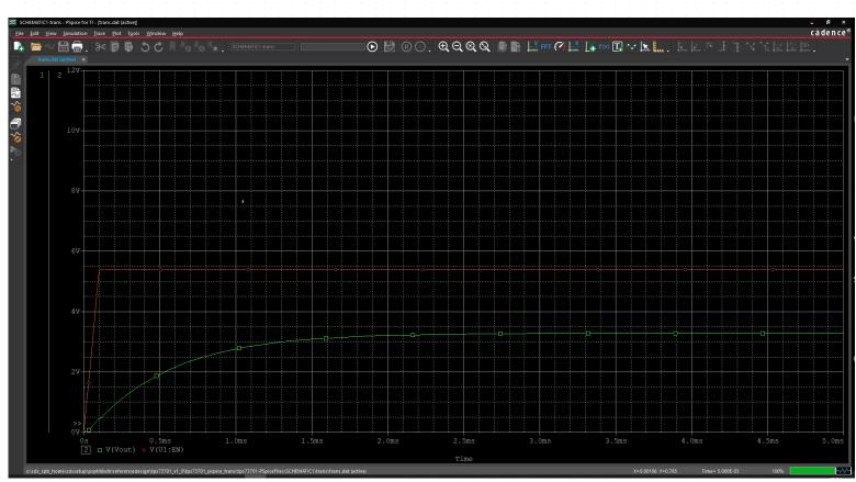
In PSpice simulation, my customer is seeing oscillation when inserting a 2.2uH ferrite bead at the input of TPS73701.
