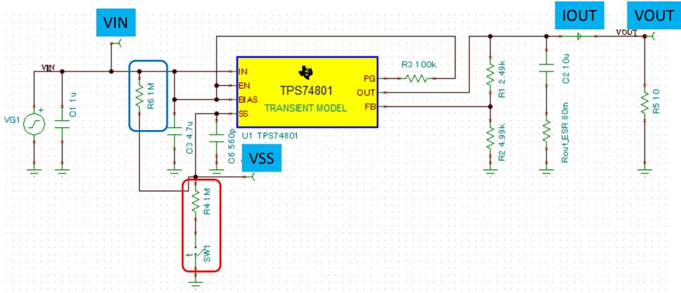
Simulate leak path from SS pin to GND due to condensation water
