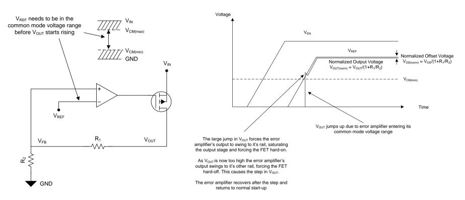
The  $V_{\text{OUT}}$  step is due to the common mode range requirement of the error amplifier
