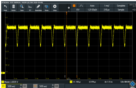
Output voltage waveform at the condition, input voltage : 3.0V, Load : 420mA
