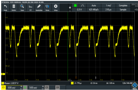
Output voltage waveform at the condition, input voltage : 3.0V, Load : 450mA
