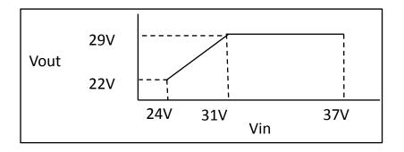
Customer wishes to automatically change the output voltage according to the input voltage.
