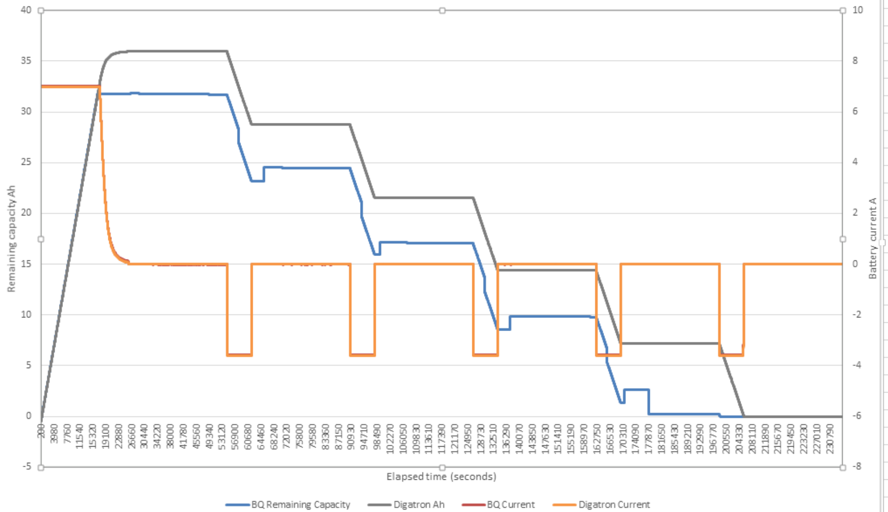
Battery A4 stepped discharge - bq / Digatron comparison - Fourth test, flag Fconven disabled 20-11-2017
