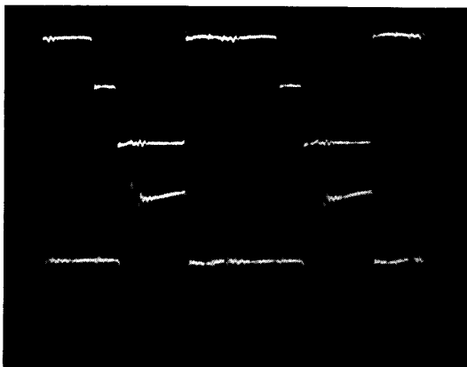
Fig. 6. Experimental waveforms. Upper trace: Drain-to-source voltage v_{ds1} . Scales: 100 V/div., 2 \mu s/div. Lower trace: Drain current i_{d1} . Scales: 5 A/div., 2 \mu s/div.
