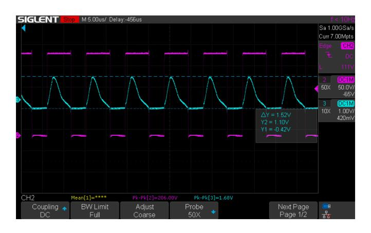
Low NV6117 Drain voltage(magenta) - 20V output RIPPLE CURRENT THROUGH RECTIFIER DIDOE (CYAN) CLOSER LOOK, EXPANDED
