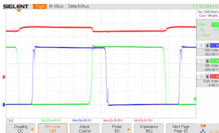
Fig 3) Typical Continuous operation of the Gate Driver
