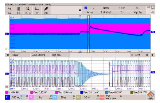
C1:5Vout[100mV/div], C2:TR5g-s voltage[5V/div], C3:TR3-gate voltage[50V/div], C4:TR3-source voltage[50V/div], Math:TR3g-s voltage[5V/div]
