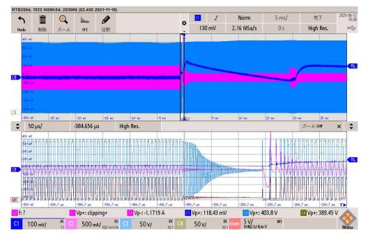
$C1:5Vout[100mV/div],\ C2:T1\ primary\ current[500mA/div],\ C3:TR3-gate\ voltage[50V/div],\ C3:TR3-gate\ voltage\ vo$
