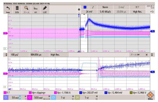
C1: 5Vout [50mV/div], C2: T1 primary current [500mA/div], C3: VCR pin voltage [1V/div],
