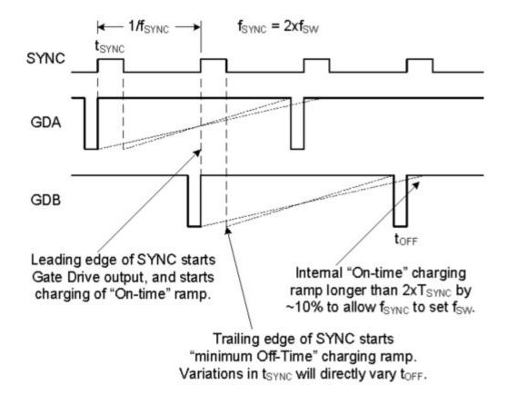
$$R_{DMX}(k\Omega) = (T_{SYNC} - t_{SYNC} - t_{OFF}) / 66x10^{-9}$$
