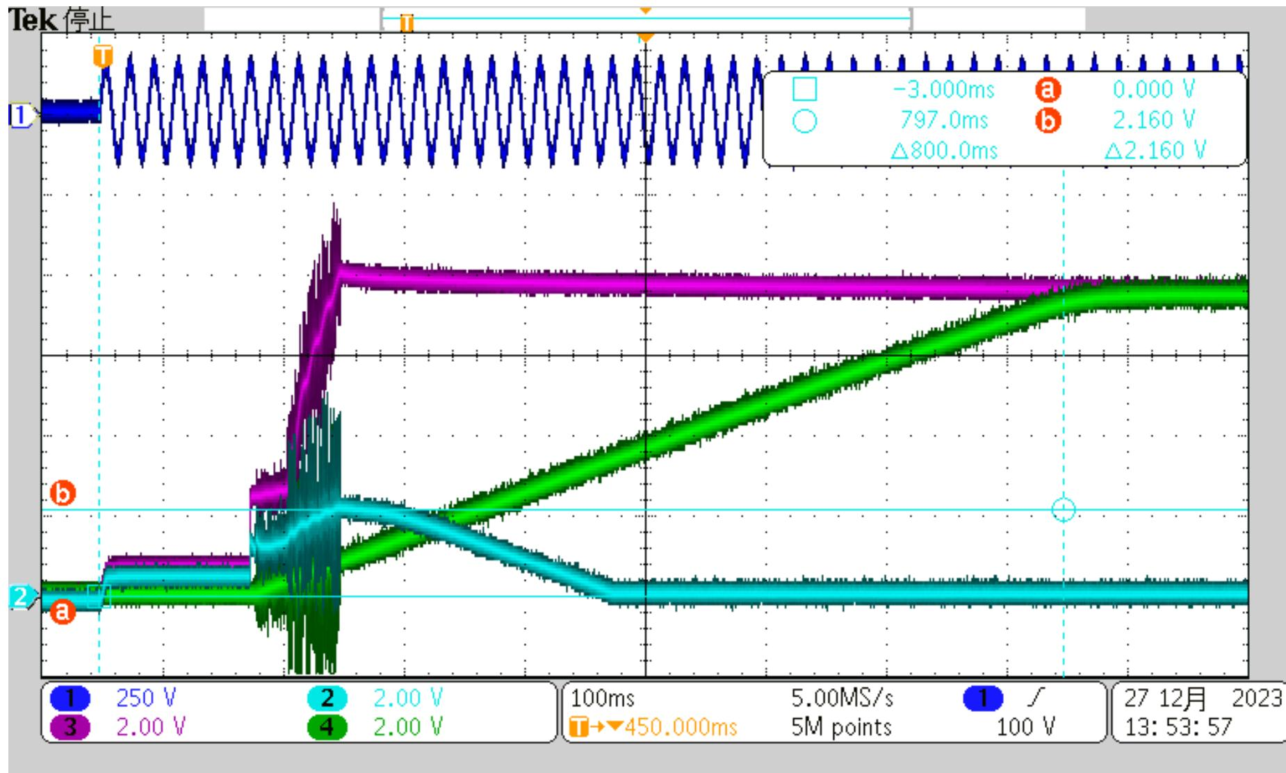
**1ch: AC Input Voltage(50Hz), 2ch: VAOUT, 3ch: OVP/EN, 4ch: SS**
