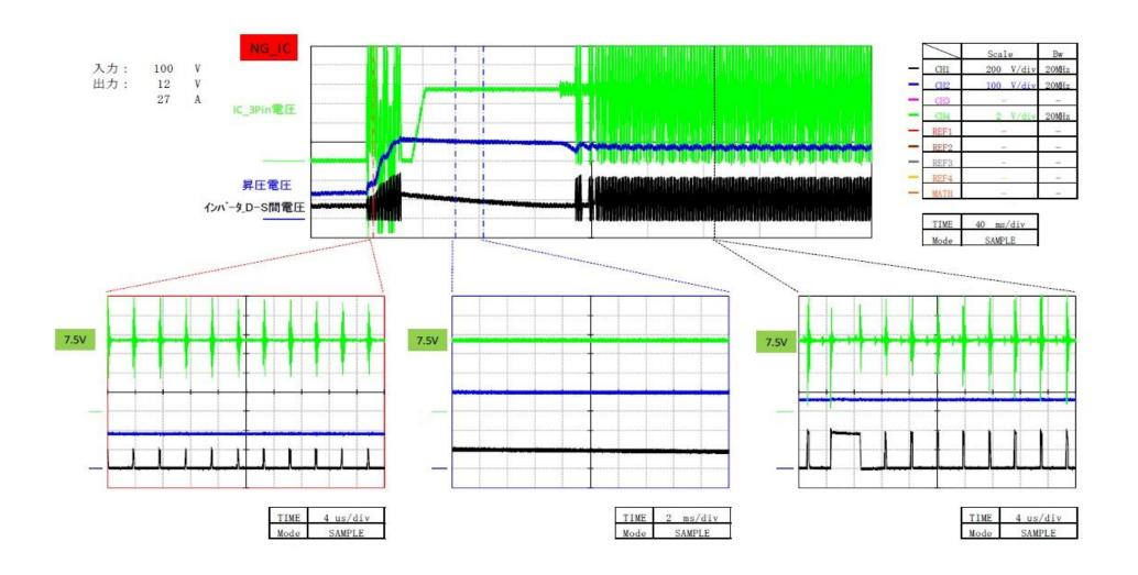
In the case of OK\_IC: When looking at the 3 pin voltage, the switch amplitude swings between 7.5 V and -2.5 V around 2 V at the time of switch operation. However, in the case of NG\_IC, it swings between 12 V and -0.5 V around 7.5 V.
