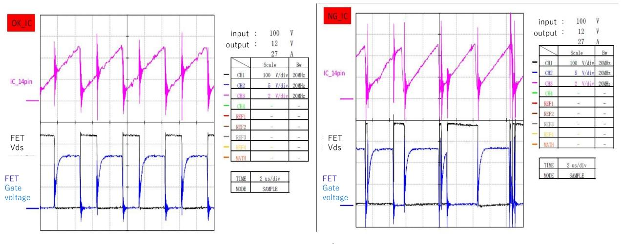
In comparison with OK\_IC, ON / OFF timing of the gate is abnormal in the case of NG\_IC.
