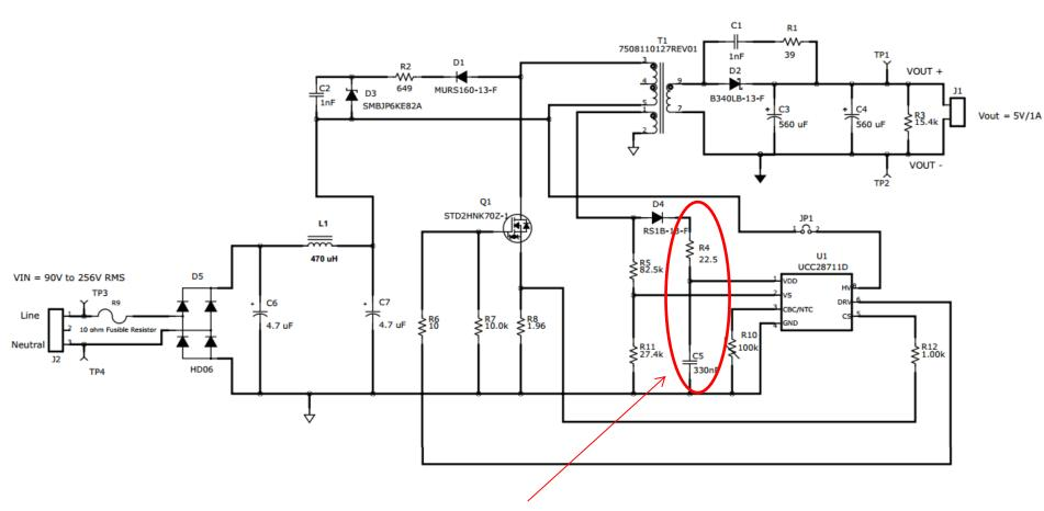
Method of determining the constants? (@22.5 $\Omega$  and 330nF)
