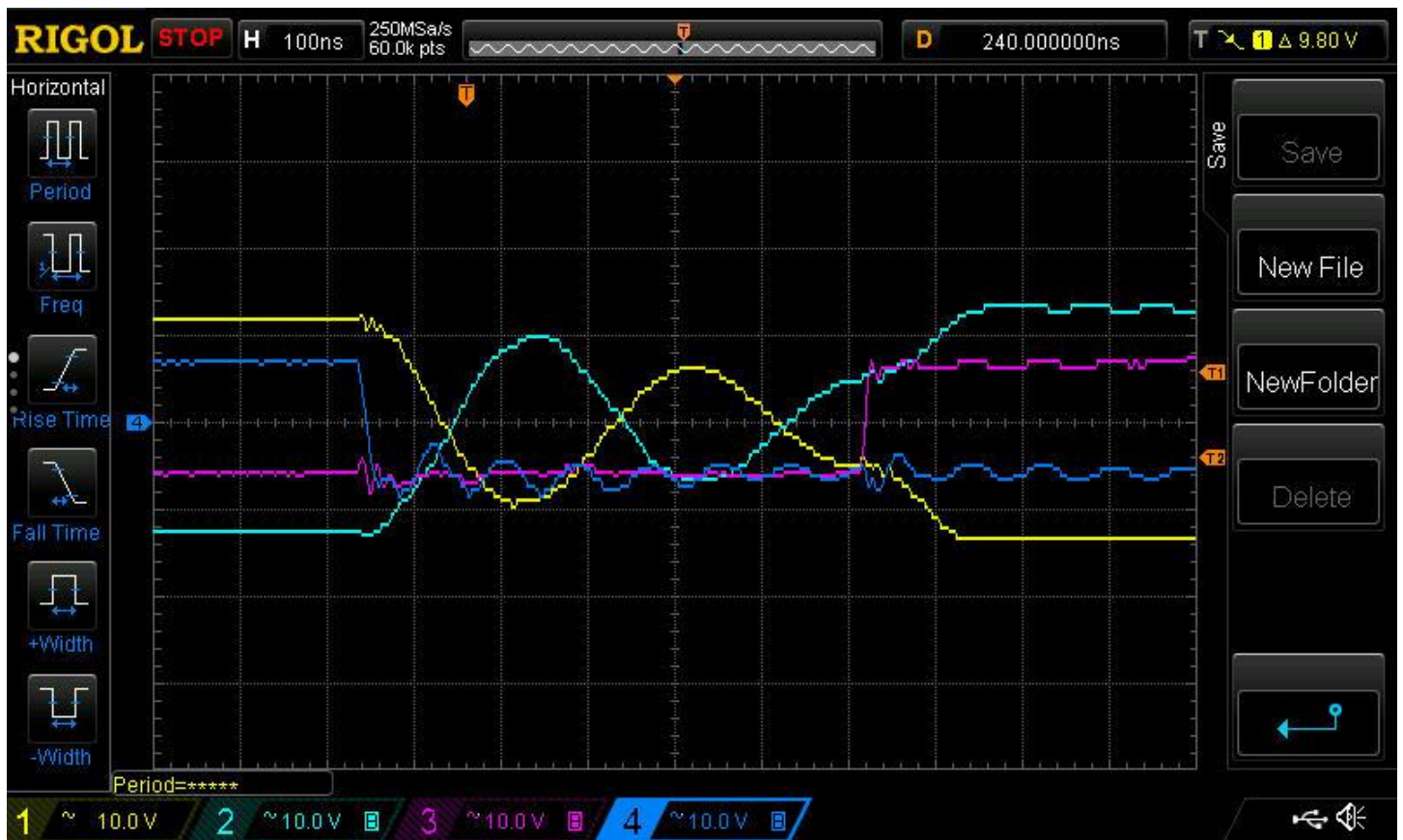
FIGURE #7 – (MAGENTA) OUTC, (BLUE) OUTD, ((YELLOW)) GDT SEC OUT #1, (TEAL) GDT SEC OUT #2 -- NO MOSFET GATES ATTACHED
