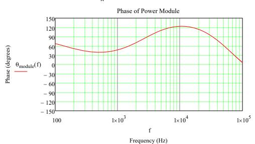
Want the total loop to cross at a decade or more befroe the module's crossover. To do this, determine what the gain of the module is at the desired system crossover frequency, determine the contribution from the open loop load share components, then select the error amplifier components to add the desired attenuation
