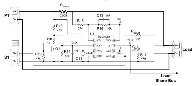
UCC29002 is enabled when VDD is greater than 4.375 V and CS- is not greater than 0.5V relative to CS+
